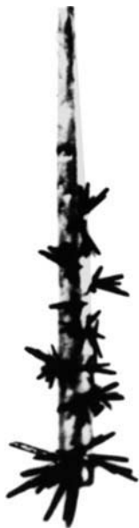
Fig. 1. [\text{Ru}(\text{bpy})_3] grown by reductive electrocrystallization on a Pt wire cathode (0.7 mm in diameter) from a solution that was 1 mM [\text{Ru}(\text{bpy})_3](\text{PF}_6)_2 in MeCN and contained 0.1 M \text{Bu}_4\text{NPF}_6 . The current density used was 11.0 \mu\text{A}/\text{cm}^2 . The photograph was taken after removing the electrode from the solution and placing it in a Schlenk tube under purified Ar.
